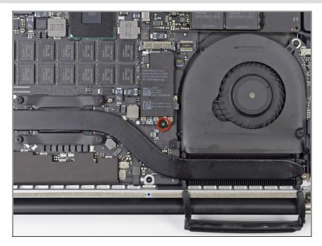
Remove the single 2.9 mm T5 Torx screw securing the AirPort card to the logic board.
